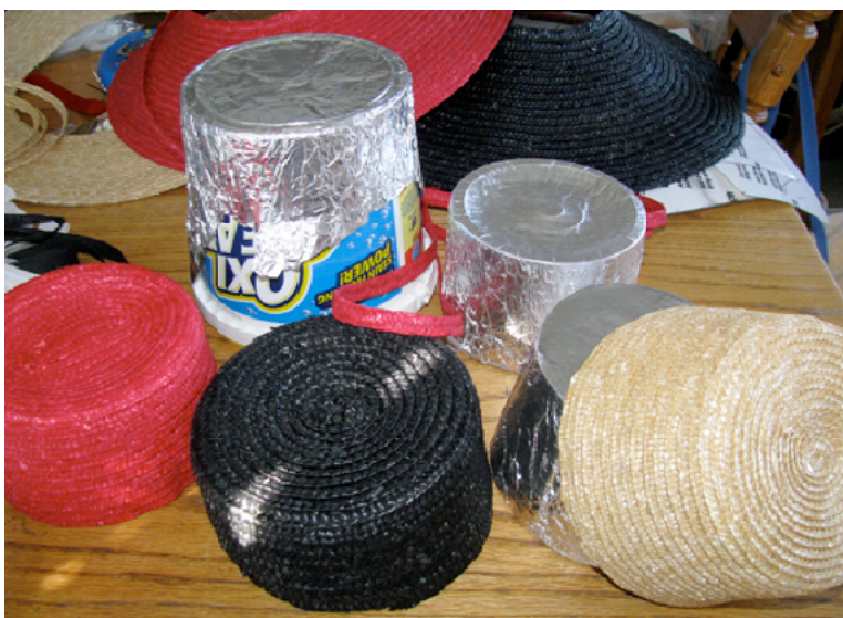
All the crowns are removed from their blocks and ready for the next step.
