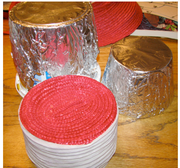
The crowns are dipped in water and stretched over their blocks. In this case they are larger around than the blocks so I need to wrap them with bias tape to cinch them in to the size and shape of the block. If these were wood blocks then push pins would be used to hold them to the base of the block.
